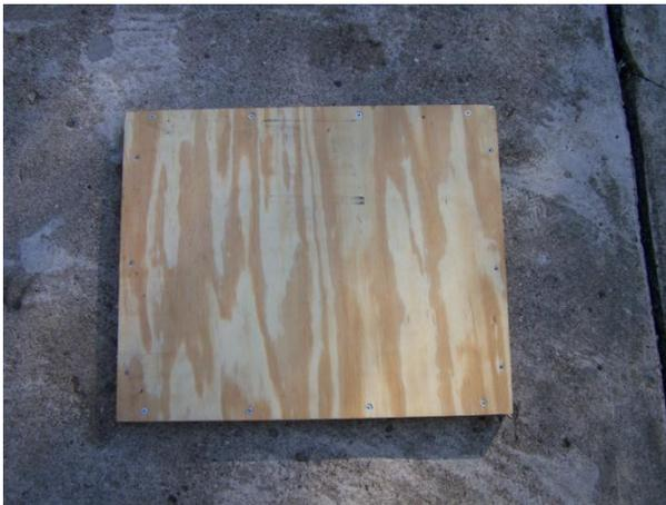
Be sure to use a short screw or nail which will secure the 1 by 2 to the plywood, but not go all the way through to the other side. 5/8ths inch screws have worked fine for me. Also, you only need enough screws to make sure pieces of the 1 by 2 boards are firmly affixed. I noticed a little overkill on the candy board depicted in the above picture. It must have been one of the first I made or the lumber was really warped. Normally you do not need 4 screws for each long side of the board.
